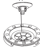
Stator with Poppet Closed
