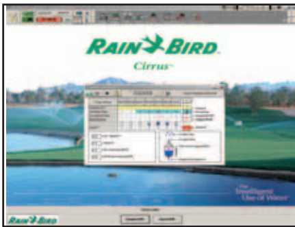
Modify irrigation schedules based on evapotranspiration rates and other Weather Station data.
